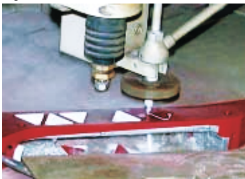
Here is the water jet making short work of blasting through the side of the riser.
